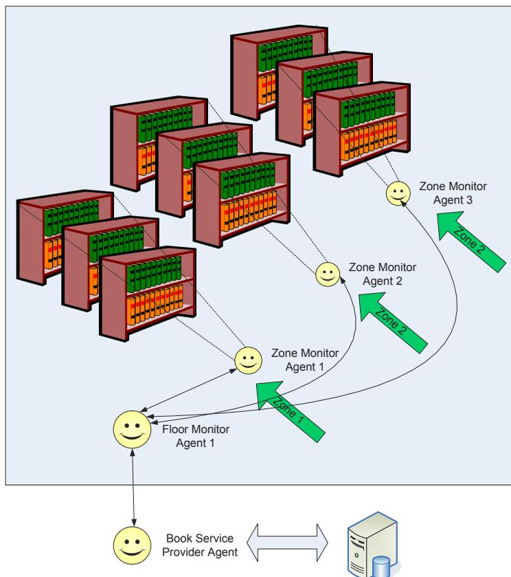
The tag embedded in each book contains information such as unique id, floor, zone, shelf, rack and availability details using a simple encryption mechanism.
